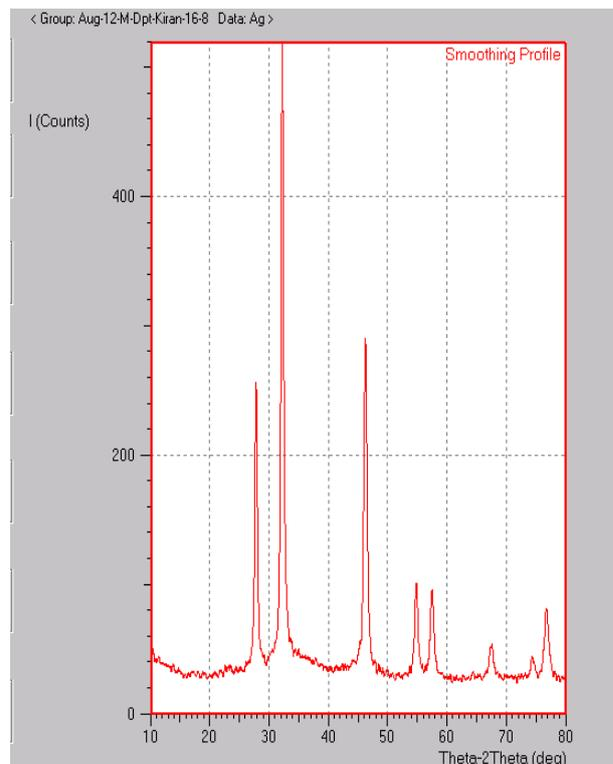
**Fig. 4. Silver nanoparticles produced by *L. amylophilus* GV6 was analysed by X-ray diffraction for identifying its nature and size.**
