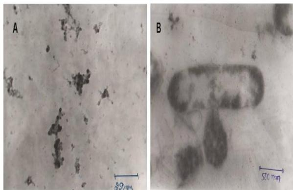
**Fig. 5. Transmission electron micrograph of silver nanoparticles produced by *L. amylophilus* GV6 for their size and location - (A) Extracellular and (B) intracellular**
