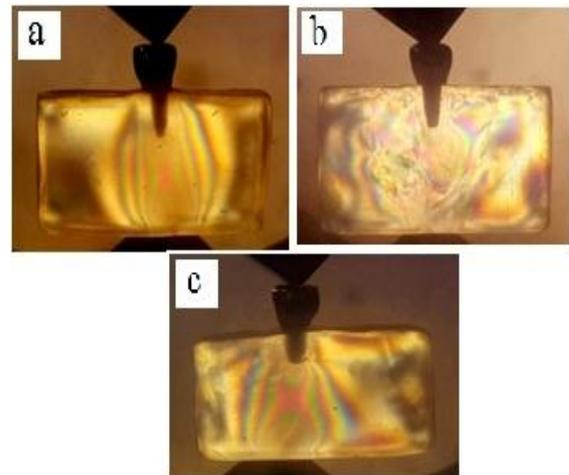
Fig 6: Group B – Axial loading with implant dimensions of a) 3.75x10, b)4.2x10, c) 5x10
