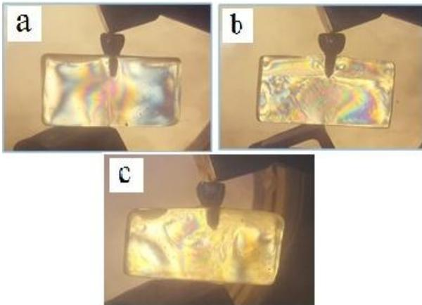
Fig 7: Group A – Oblique Loading with implant dimensions of a) 3.75x10, b) 4.2x10, c) 5x10
