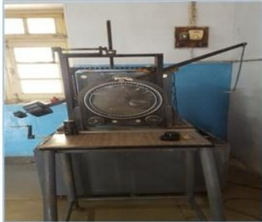
Fig.4 circular polariscope
