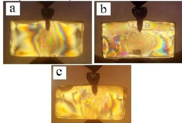
Fig 5: Group A – Axial loading with implant dimensions of a) 3.75x10, b) 4.2x10, c) 5x10
