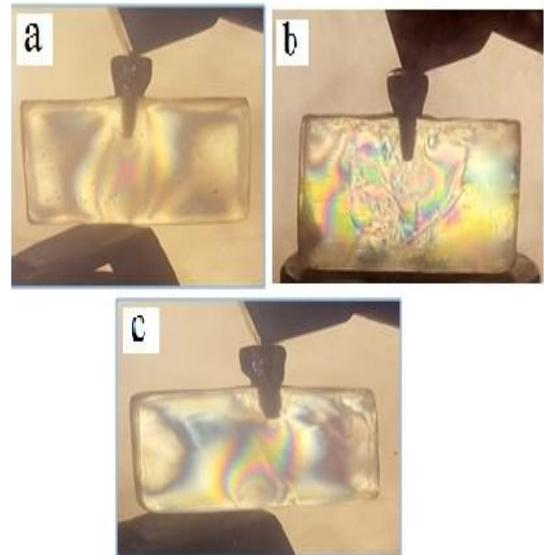
Fig 8: Group B – Oblique Loading with implant dimensions of a) 3.75x10, b) 4.2x10, c) 5x10
