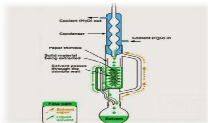
Fig. Soxhlet extractor
