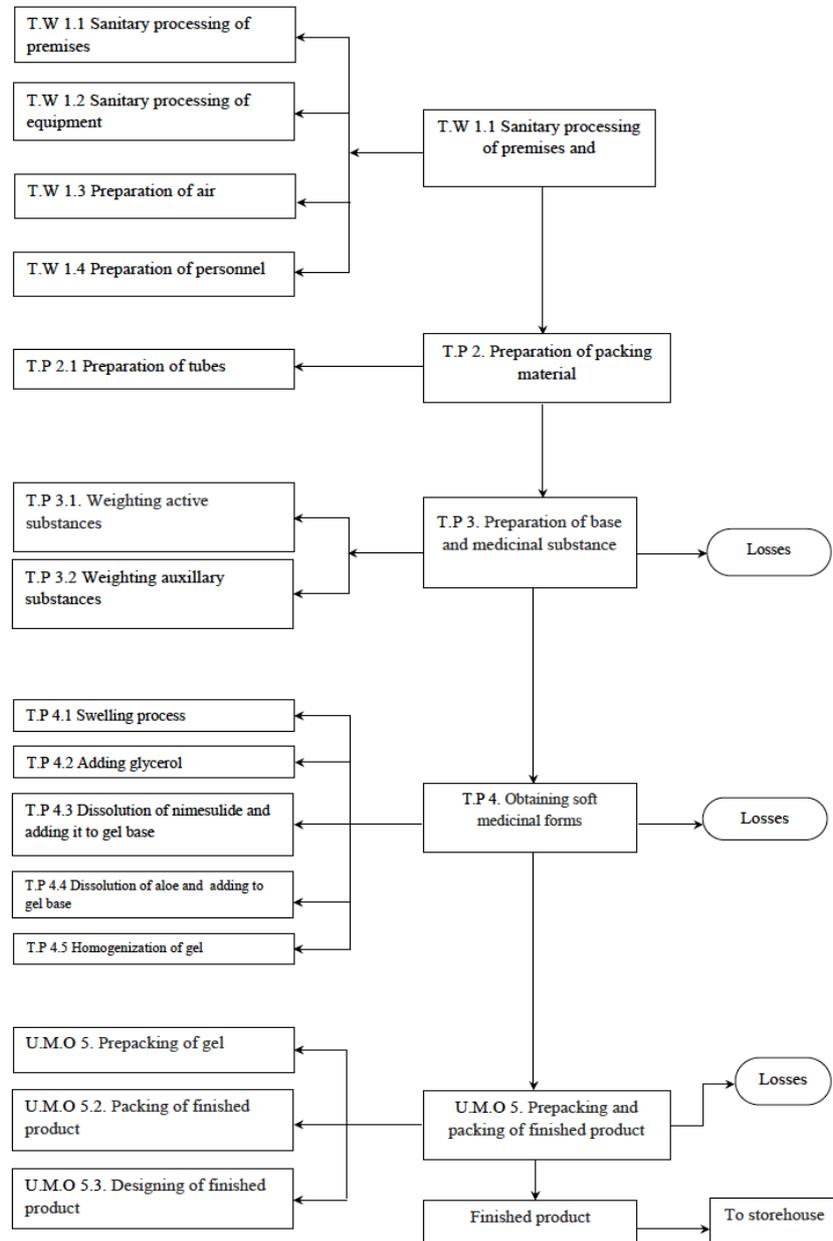
**Fig. 1: Technological scheme of production Alnident gel**
