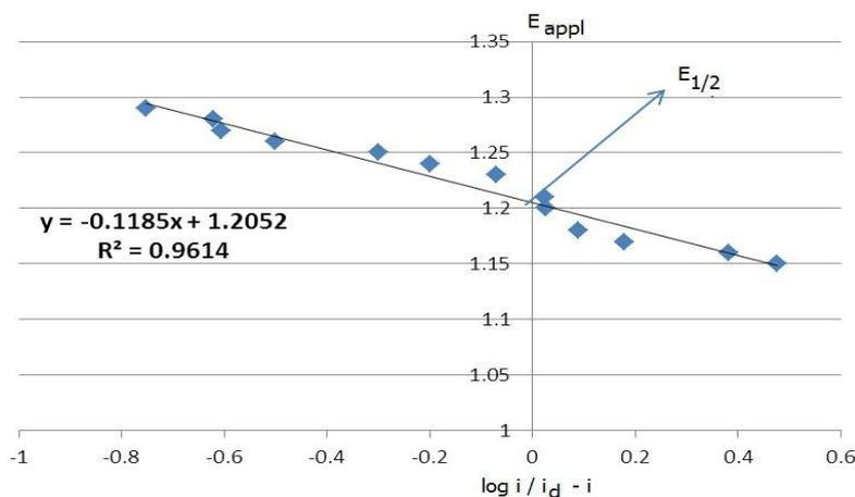
**Figure 4: Effect of E applied on the  $\log (i/i_d - i)$  variation using Heyrovsky-Ilkovic equation at  $0.8\mu\text{g.ml}^{-1}$  Meloxicam concentration.**
