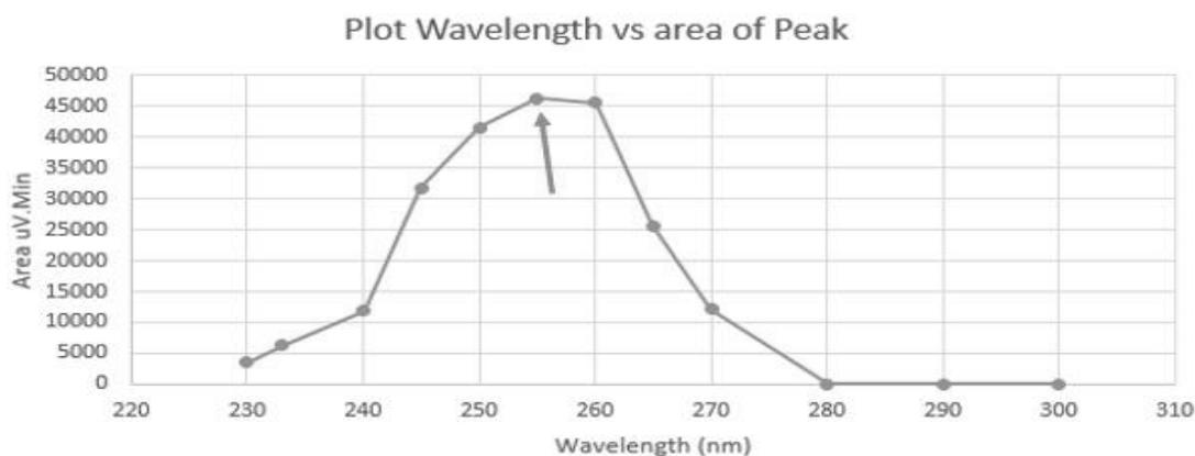
**Figure 2:** Absorbance spectra of ephedrine alkaloid from 300 nm to 230 nm. The optimum absorbance value occurs at 255 nm. Mixture is 0.04497 molar ephedrine alkaloid in 10% ethyl alcohol (v/v) and 90% distilled water.
