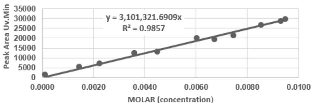
**Figure 3:** Standard curve for determination of ephedrine alkaloid. Equation of line is  $y = 3,101,321.6909x$ , with coefficient of determination at 0.9857, indicating that molar concentration accounts for 98.57% of the variance in peak area. Pearson r correlation is 0.9928 indicating very strong positive relationship.
