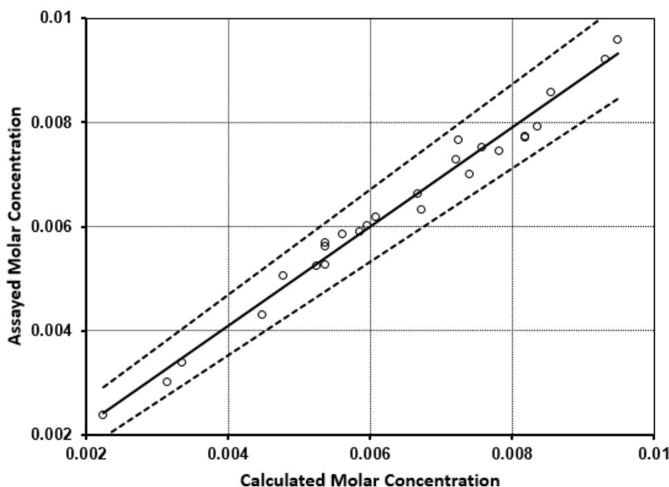
**Figure 4: Passing-Bablok plot of calculated molar concentration values compared to values of molar concentration values obtained from assay by HPLC. Value of 1 is contained within the 95% confidence interval of the slope (0.8970 to 1.0113). The value of 0 is contained within the 95% confidence interval of the y-axis intercept (0 to 0.007). Pearson r correlation is 0.9913, with no departure from linearity by applying “runs test” ( $P=.08$ ).**
